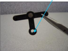
Apply one drop of Glue (supplied with Escrow Arm) inside the Shaft Hole on the back of the new Escrow Arm
