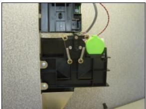
Align flat spot in Shaft Hole with flat spot on Shaft and press new Escrow Arm in place until Shaft is flush with front of new Escrow Arm.
